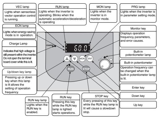
Fig. 33 — 50BV VFD Display
